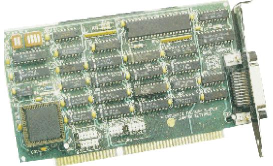
The OMEGA OMB-PER488/AT converts IBM PC/XT/AT and compatible computers into highperformance IEEE-488.2 compliant controllers. The board reads data at up to the 1 Mbyte/sec maximum specified by the IEEE-488 bus. This high-speed throughput is achieved with special circuitry that combines two 8-bit IEEE data bytes into a single 16-bit word for DMA transfer on the 16-bit AT bus.
